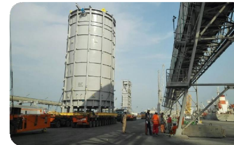
RADIANT MODULE RM-01 Dim: 10.00 * 8.90 * 17.00M (LWH) GWT: 196.00 tons
