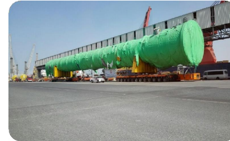
DEISOPENTANIZER Dim:83.8 * 8.62 * 9.87M (LWH) GWT: 480 tons
