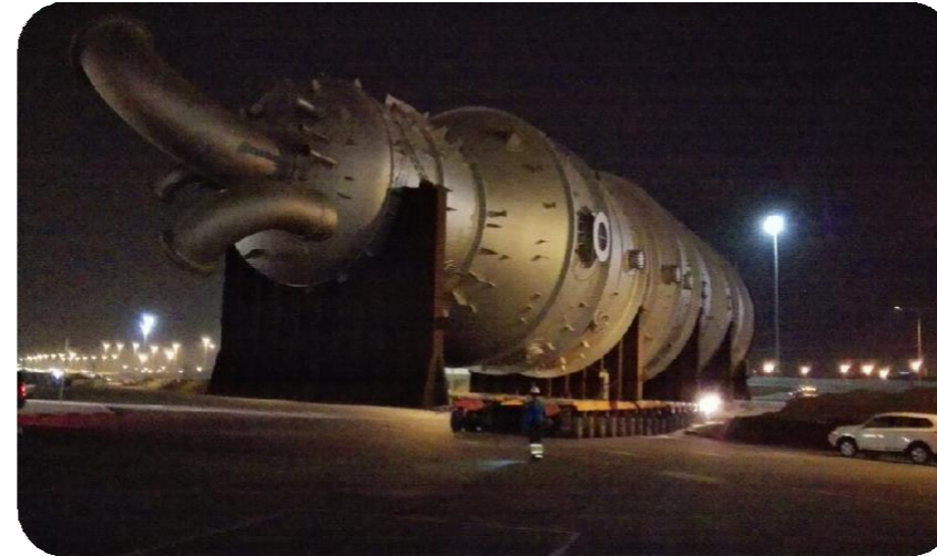
VACUUM COLUMN Dim:60.10 * 10.80 * 10.95M (LWH) GWT: 535 tons
