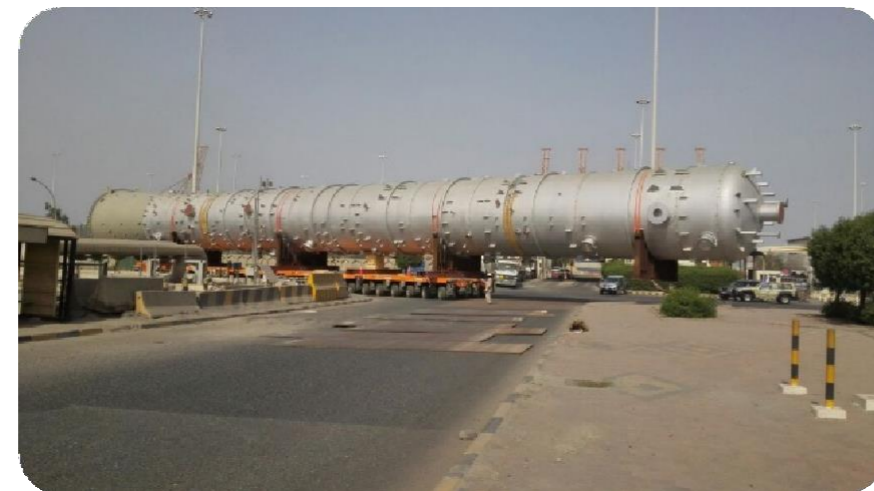
COKER FRACTIONATOR Dim: 65.30 * 7.30 * 7.90M (LWH) GWT: 327 tons
