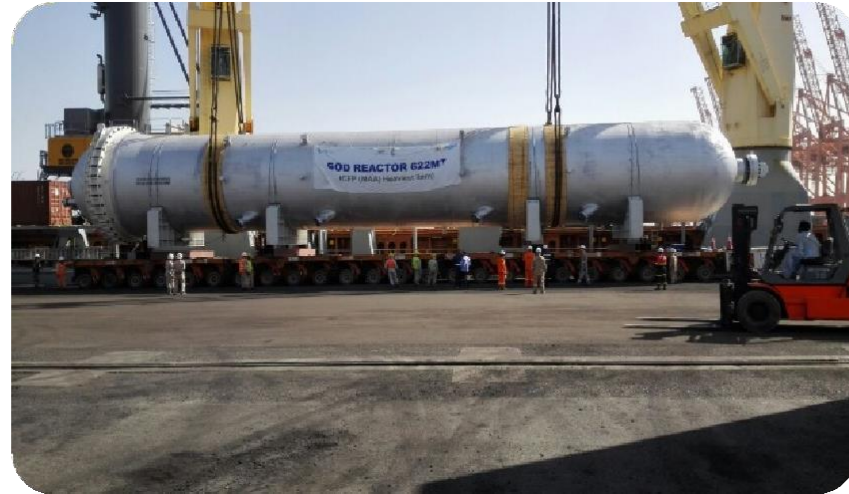
GOD REACTOR Dim:38.47 * 6.46 * 6.58(LWH) GWT: 622 tons
