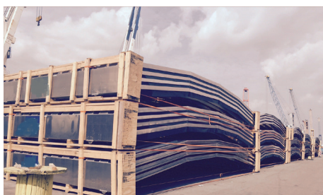
Innovative packing design allowing 3 tier high stacking
